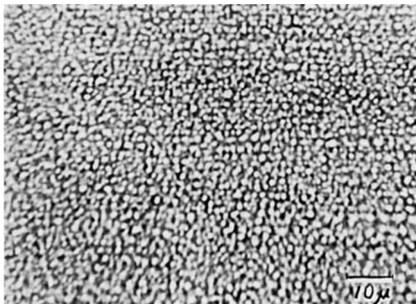
Fig. 5. O/W type emulsion of unsaturated polyester resin. [TEA] = 0.24 mmole/g.
